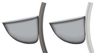
Thick side of the belt is facing pulley
